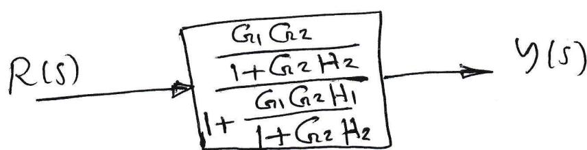
the transfer function  $\frac{Y(s)}{R(s)} = \frac{G_1 G_2}{1 + G_2 H_2 + G_1 G_2 H_1}$
