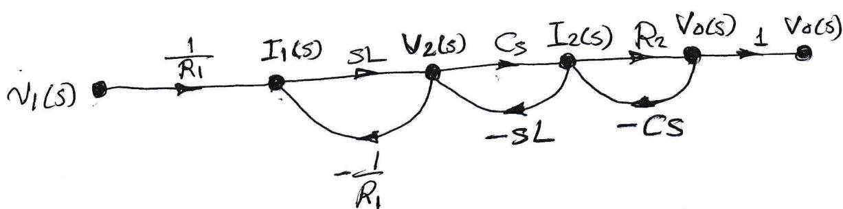
EX obtain the signal flow graph for figure below
