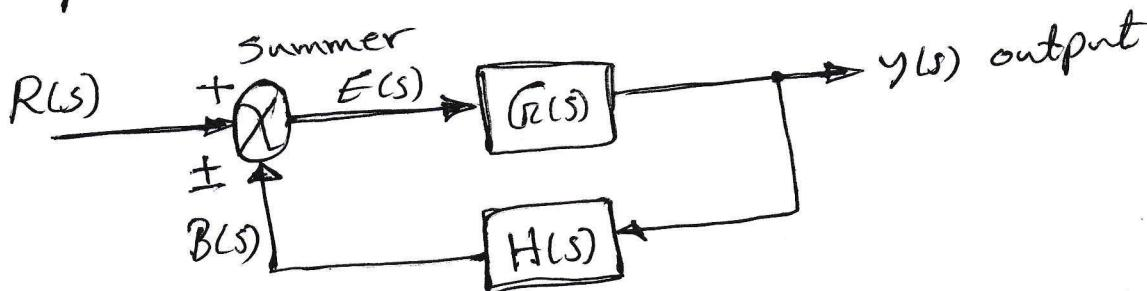
$\underline{G(s)} = \frac{y(s)}{E(s)}$  : Forward path transfer function or plant transfer function.
