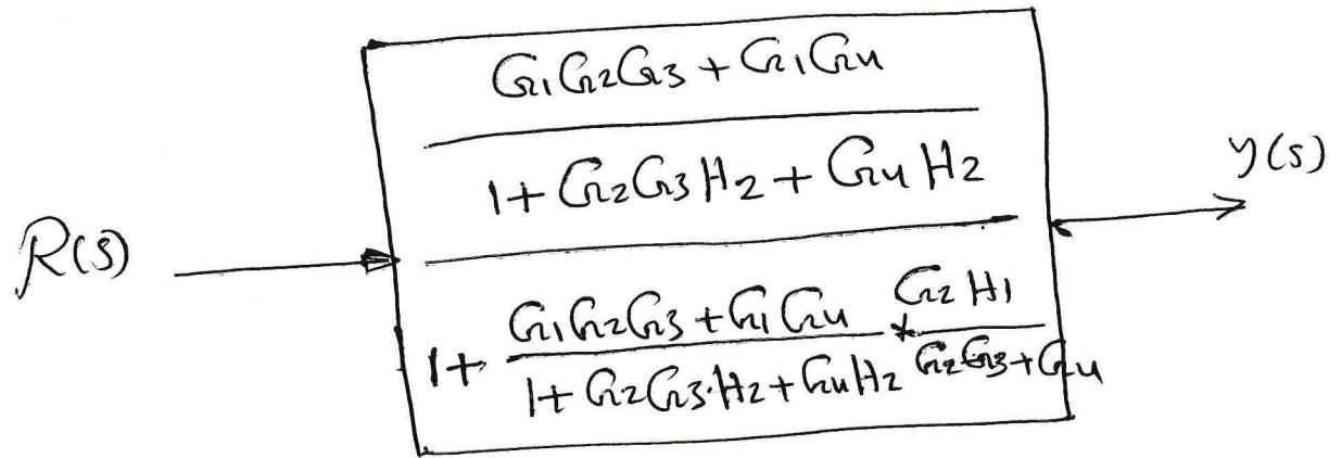
$$\therefore T-f = \frac{y(s)}{R(s)} = \frac{\cancel{G_1G_2G_3 + G_1G_u}}{1 + H_2(G_2G_3 + G_u) + H G_1G_2}$$
