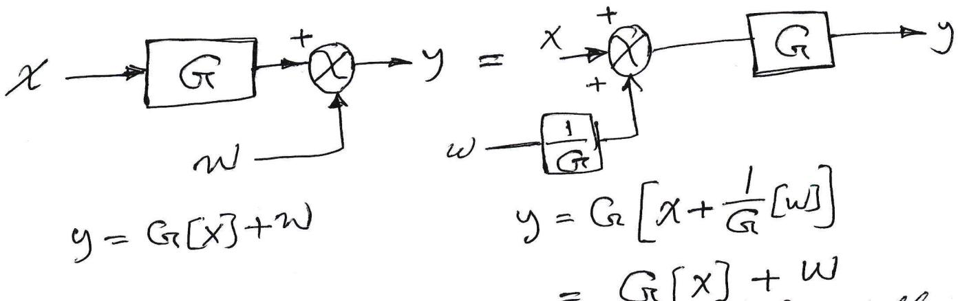
Rule 3 :- A summing point can be moved from left side of the block to right side of the block.
