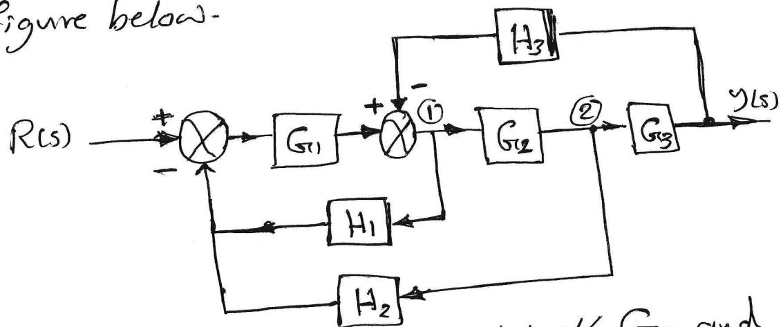
① moving point (2) to the right of block  $G_3$  and combining blocks  $G_2$  and  $G_3$ .
