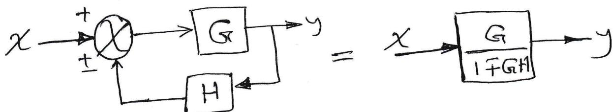
Ex Find the overall transfer function of the system  $\frac{Y(s)}{R(s)}$  in figure below, using block diagram reduction technique.
